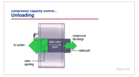
As the slide valve continues to open, further unloading the compressor, its radial discharge port eventually travels past the opening in the compressor housing. Once this occurs, all of the refrigerant vapor being pumped by the compressor is discharged through the axial port in the compressor's end-plate.
